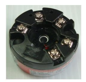
The Model LW-242 is an analog, isolated 2-wire head-mounted temperature transmitter that converter the thermocouple input into a proportional to the voltage generated by the thermocouple sensor, linear, and highly accurate 4- 20 mA output current in a variety applications such as process control, automation system, and energy source management.
