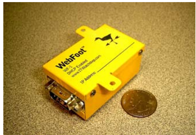
The small tabs provide an easy way to attach the WebFoot to a wall or a bracket. No special mounting considerations are needed. The metal case is powder-coated for durability.
