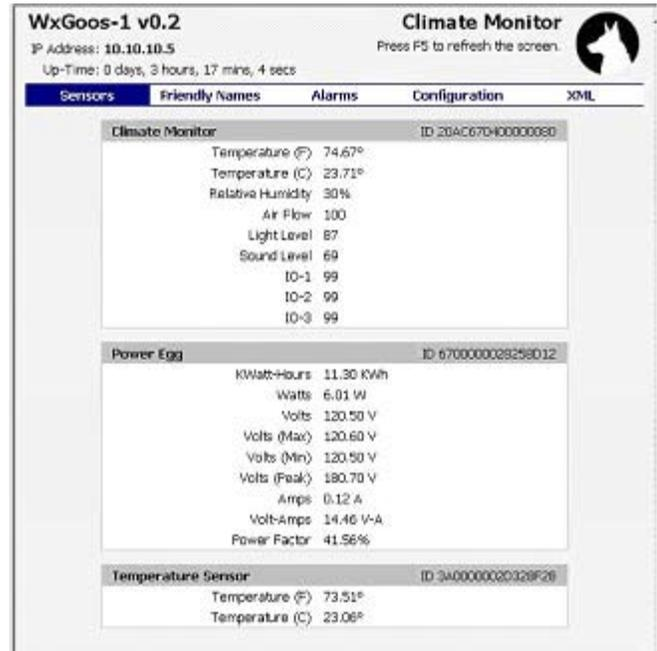
The picture shows a typical web presentation of a cabinet. Both real-time data and a history (in this case six days) can be seen. When new remote sensors are detected, they are added automatically to the web page display.
