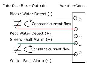
When the WaterSnake is configured in the Supervisory Mode, as shown above, the relays are in a constant closed state. If the power should fail or the cable become disconnected, an alarm will be sent.
