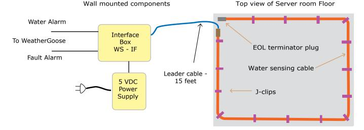
The WaterSnake's four components: the sensing cable, a leader cable, the interface box and a small power supply. The interface box and power supply are usually wall mounted. The sensing cable secures to the floor with plastic J-clips.
