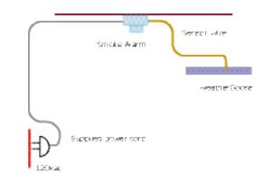
The supplied wiring makes installation easy. Plug the cord into the wall plug; attach the output wires into the WeatherGoose. Test the installation by pressing the alarm's Test button.
