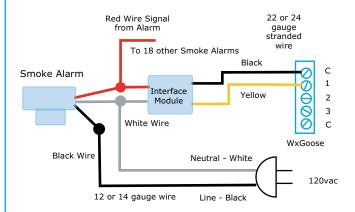
The schematic shows how the Smoke Alarm wires to the interface and the WeatherGoose. Up to three can be directly attached to the three C123C ports on the Gooses and the Duck.
