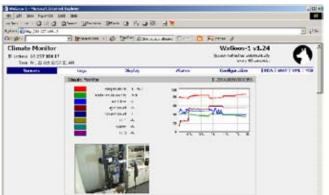
A web page displays the current values with graphs showing trends. The web cam image is JPEG format. The data can be viewed on a PDA and cell phone. The unit is configured via the web page. The web page can be quickly configured to specific logos and brand names.
