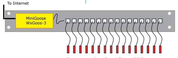
Temperature, humidity, airflow or CCAT sensors
