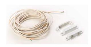
The sensors mount in two parts; the switch body (the part with the screw terminals) and the magnet. These should be mounted as close as possible. The range of operation is about an inch. The third part is a plastic screw terminal cover.
