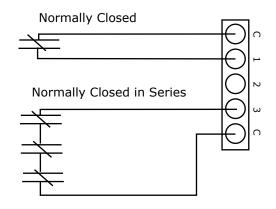
Connect the sensors to the C123C block. "C" is common (ground). If more than three door sensors are to be used, they can be wired in series (Normally Closed). When one opens, the current ceases and a alarm is sent. If Normally Open sensors are used they should be wired in parallel.
