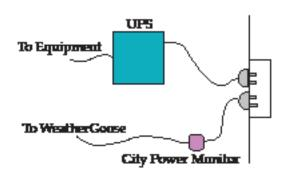
The CPM must be connected directly to a receptacle supplying city power and not to the UPS power. Graphs will show loss of city power.
