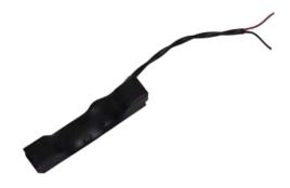
Each end of the CCAT is an RJ-11 receptacle. The twisted pair receives the analog signal input.
