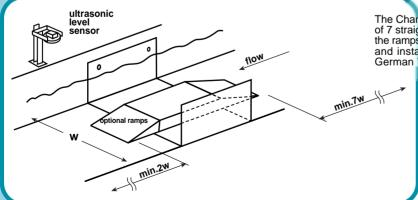
The ChannelMag CM2 accuracies are based on a minimum of 7 straight channel widths (7W) upstream (from the end of the ramps if supplied) and 2W downstream The ChannelMag and installation conforms to the German DIN 19559 and German Waste Water Institute (ATV Arbeitsgruppe 1.2.5).
