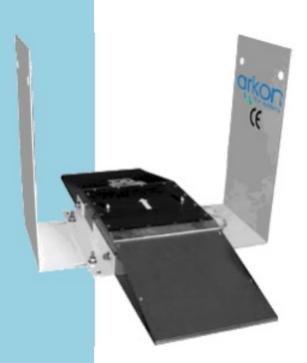
The ChannelMag is a bi-directional magnetic flowmeter system, suitable for use in existing channels of various shapes from widths or diameters 6" - 200 feet (150mm to 60m). It is suitable for raw sewage or storm water. The electrodes may be permanently coated with sewage grease, algae, and calcium carbonate or similar, without the need to clean.
